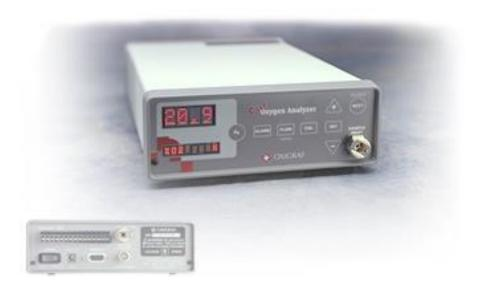
The Model O2 is a versatile research grade oxygen analyzer for measuring 5-100% oxygen concentrations. The unit features an easy to use and feature bright LED displays, touch panel controls, easy calibration, and a CPC front panel fittings. The Model O2 has a built-in sampling pump, flows of 50 or 150 ml/min may be selected via the front panel keypad.
