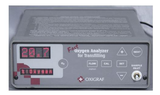
The Model O2T oxygen analyzer for medical oxygen trans-filling and verification is designed for measuring 5-100% oxygen in nitrogen. The unit features an easy to use and feature bright LED displays, touch panel controls, easy calibration, and a CPC front panel fittings. The Model O2T has a built-in sampling pump with flow from 0-250ml/minute.
